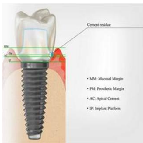
Figure 1: Section of cement-retained implant-supported prosthesis showing reference points used to calculate distances. Cement residue is represented in blue. AC: Apical Cement; IP: Implant Platform; MM: Mucosal Margin; PM: Prosthetic Margin [8].
