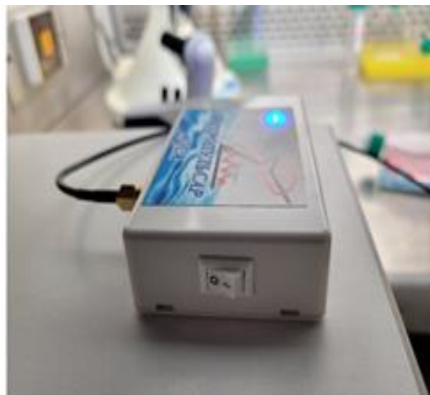
Figure 2: Operating modes of the Synchropulsar Aqua device. Left: Power toggle is in pose turn on; Right: Switch of dual mode is in the position continuous generation.
