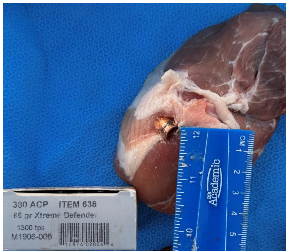
Figure 8: The Underwood Xtreme Defender projectile stuck in the most distal muscle of the chest model.
