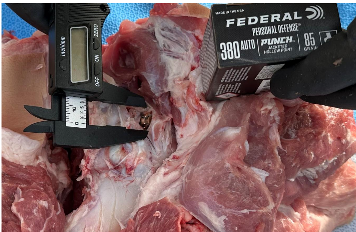
Figure 4: Federal JHP stuck inside the bone
