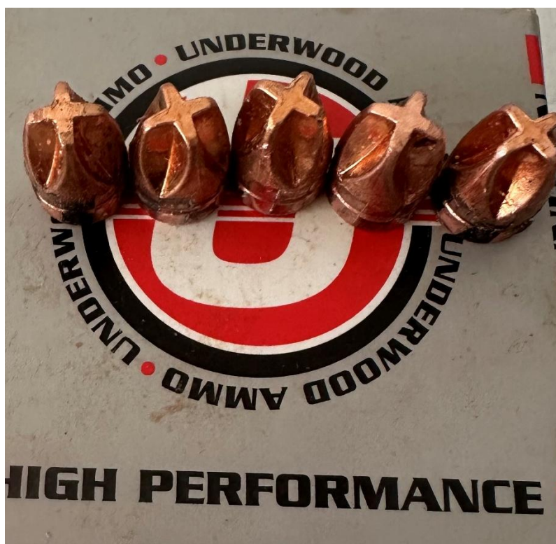
Figure 6: Copper alloy projectiles from Underwood Xtreme Defender penetrated without any deformation or fragmentation.
