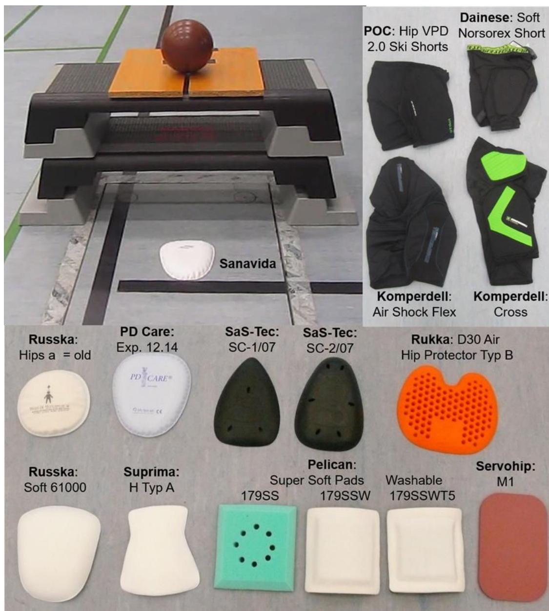
Figure 3: The hip protectors shown here (and also a 60 mm thick Airex mat, see Fig. 4) were placed on a Kistler measuring plate and a 3.1 kg bowling ball was dropped from heights of 25 cm, 45 cm, 65 cm, 85 cm and 100 cm.
