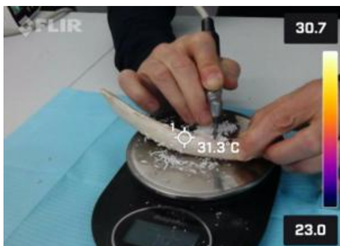
Figure 4: An electronic scale was used to measure the constant force applied on the drill bit by the user.
