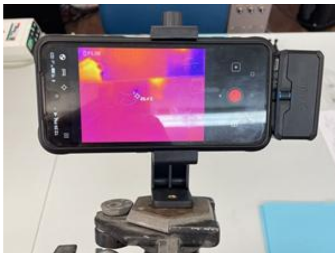
Figure 3: Flir One Pro LT thermal-vision camera (tolerance \pm 2^{\circ}\text{C} ) mounted on a solid tripod used to measure the bone and the drill temperature [10].
