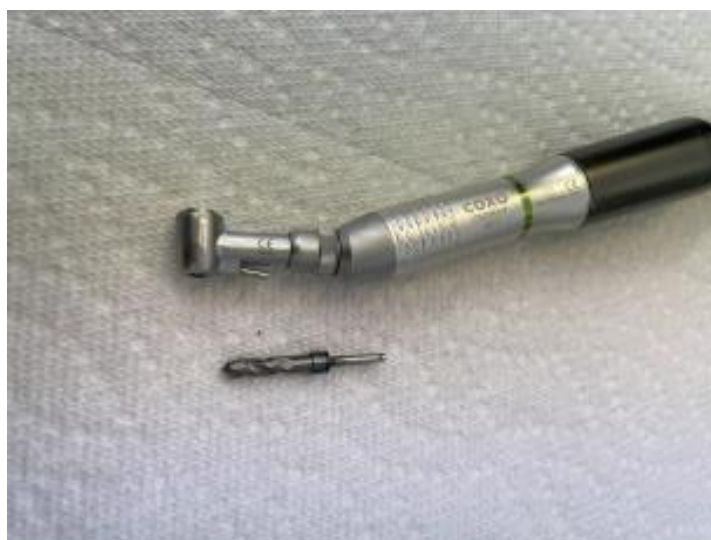
Figure 2: A 4 mm, high thermal conductivity drill. The drill was driven by a Dental surgical micro- motor equipped with a 20:1 re- duction implant contra-angle handpiece.
