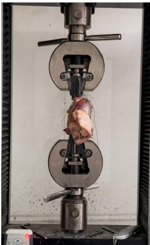
Figure 2: Specimen mounted onto a micro universal testing machine.
