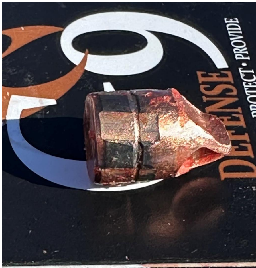
Figure 11: The G9 solid copper fluted projectile completely intact after penetrating through the combined biological specimen i.e. the shoulder model and the chest model. It was retrieved from the copy paper backstop.
