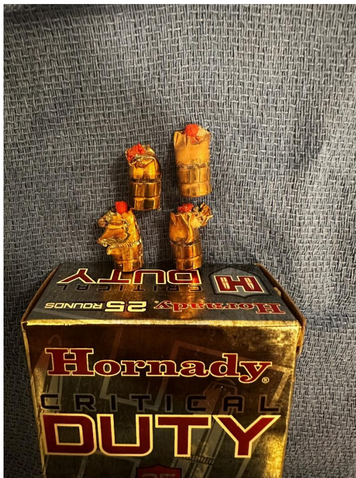
Figure 13: Here are 4 examples where no expansion occurred. Clogging with a soft material took place. Smooth expansion did not take place when hard surfaces were met.
