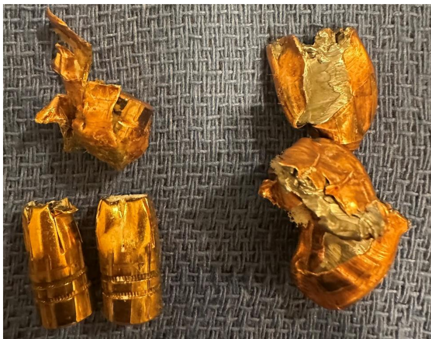
Figure 9: JHP ammunition from different manufacturers all show the same pattern i.e. non expansion and even closing up after contact with hard objects.
