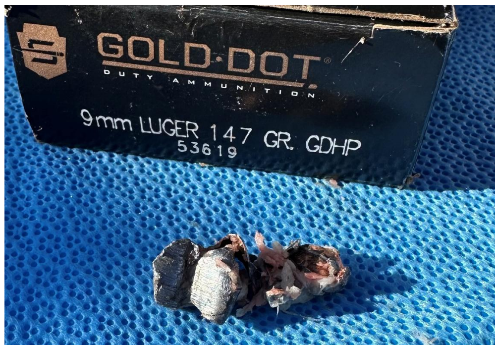
Figure 2: This is an example of a JHP that penetrated through bone. It fragmented and lost some of the petals. This is typical for a JHP through bone. It does not demonstrate the smooth projectile expansion of muscle penetration.
