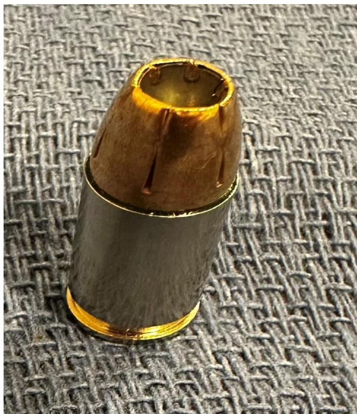
Figure 3: Federal HST an example of a jacketed hollow point with a copper jacket and a lead core.
