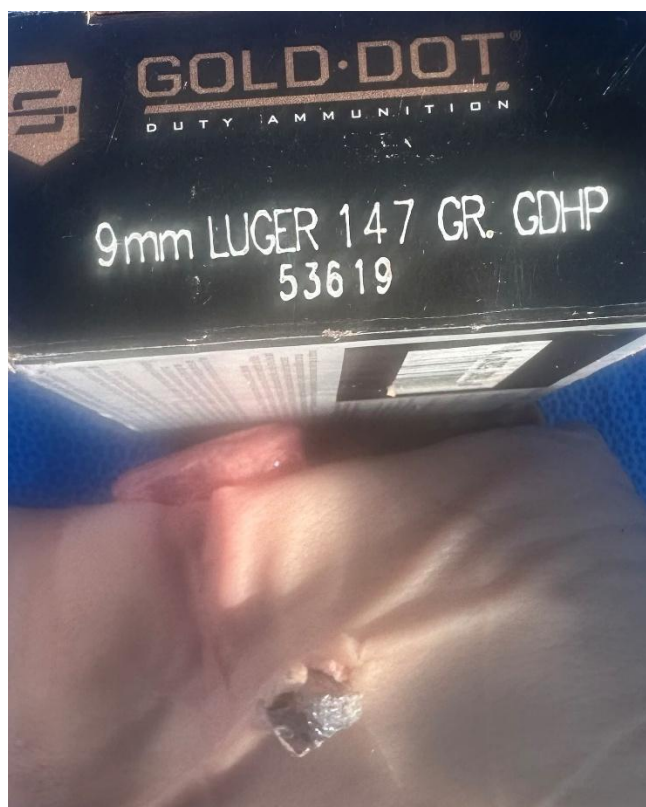
Figure 5: The projectile got stuck in the chest model. This is an example of a projectile that penetrated through the chest model including the humerus but did not have enough momentum to exit the chest model and therefore did not penetrate the chest model at all!
