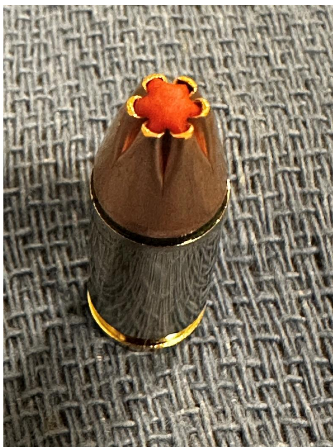
Figure 4: Hornady Critical Duty: a Jacketed Hollow Point with a red plastic plug to prevent clogging with clothing fibers.
