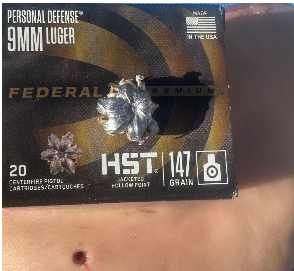
Figure 7: An example of the Federal projectile recovered after passing through soft tissue only. It shows perfect expansion of the jacket but with an intact central core as advertised on the box. This does not represent a projectile that penetrated bone.
